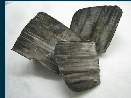
Lithium is required for production of  $^3\text{H}$  (tritium) in the fusion plant
